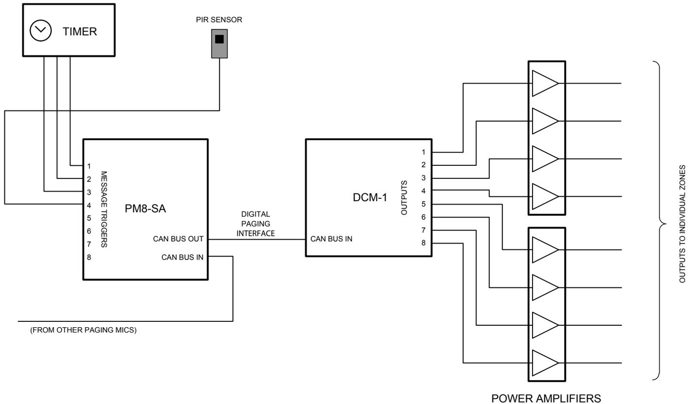
The example shows a PM8-SA connected to a DCM-1 Digitally Controlled Mixer via the Digital Paging Interface. The interface is a single CAT-5 cable which carries power, audio and zone selection commands. Other PM paging microphones (elsewhere in the building) may be daisy-chained to the PM8-SA with further single runs of CAT-5, and all microphones can access all the DCM-1's zones, if wished.
