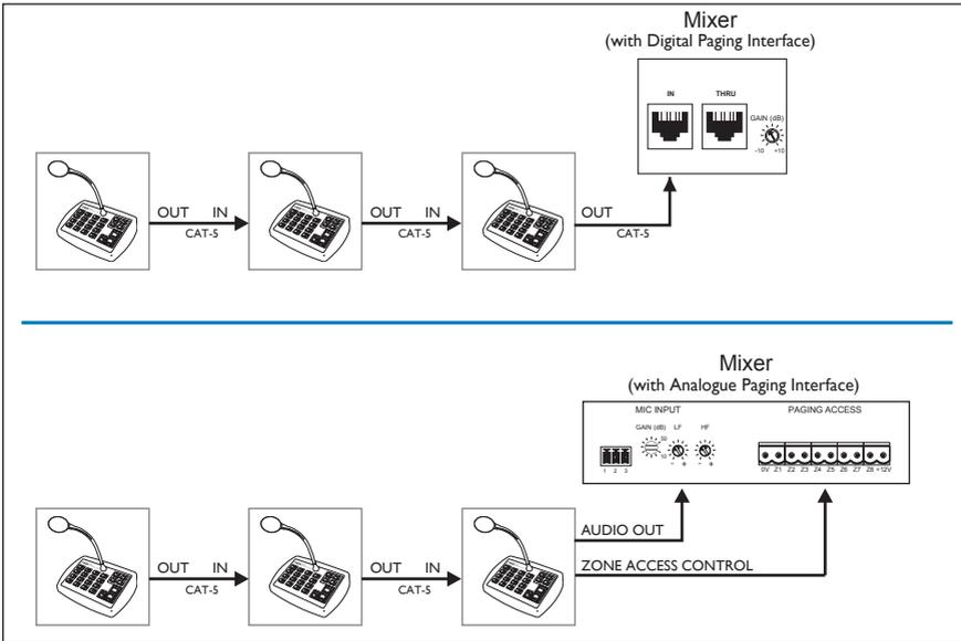
Note that there is no restriction as to the PM model which is the 'last' in the chain – i.e., that which connects directly to the mixer. All PM models support all 16 zones, so in an extreme example, several PM16s could be daisy-chained with a PM4 as the 'last' microphone in the chain. All microphones on the system will have full access to whichever zones are required.
