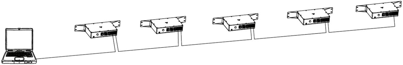
If more than five (5) devices are required, a one-gigabit ethernet switch may be used to expand the size of the network. However, even in this case, no more than ten (10) branches from the ethernet switch are allowable, with each branch containing up to five (5) daisy-chained devices. This permits a maximum of fifty (50) devices to be linked to a single controller, as shown in the image below.
