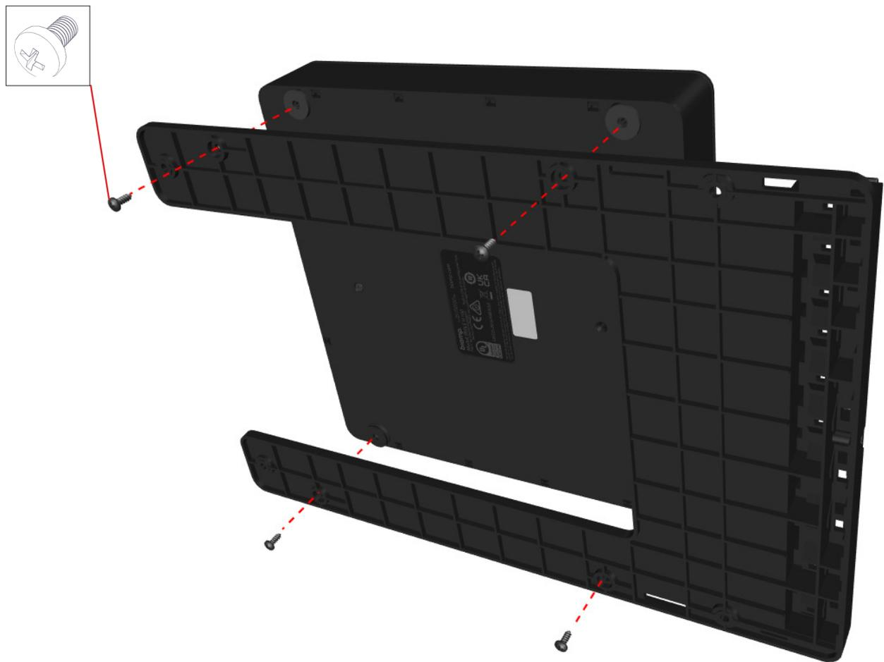
2. Unscrew the four screws attaching the bracket to the bottom of the device.
