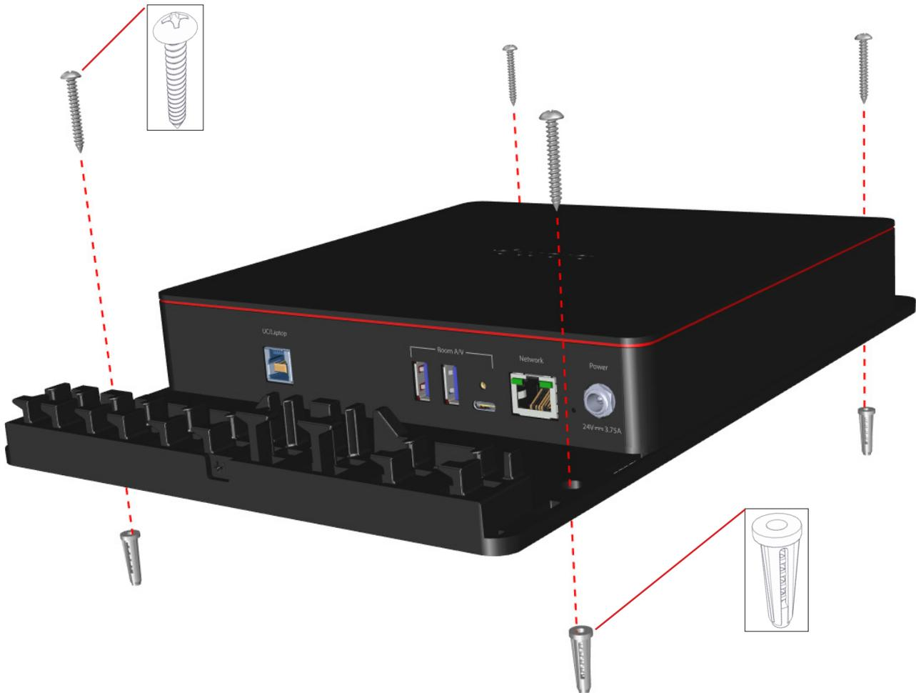
3. Use the four holes on the mounting plate to mark the locations for the wall anchors and screws.
