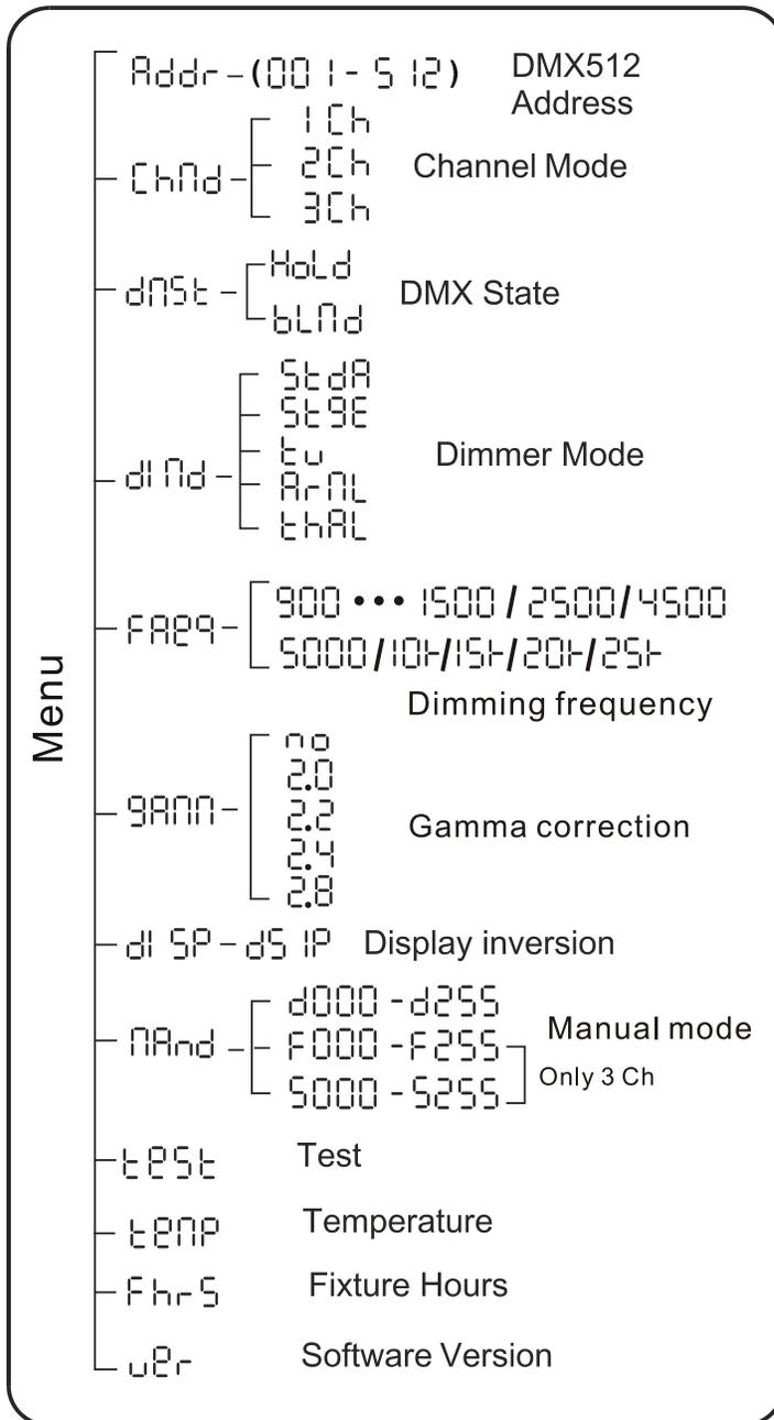
**System Menu:** When making adjustments press **ENTER** to confirm your setup then press and hold the **MENU** button for at least 3 seconds. To exit without making any adjustments press the **MENU** button. The display will lock after 30 seconds, press the **MENU** button for 3 seconds to unlock.
