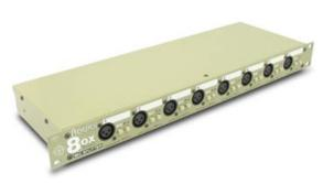
The Radial 8ox is a 19" single space rackmount 8 channel mic splitter that has been designed to provide a compact and efficient method of taking 8 microphones and splitting the signal to a recorder and public address sound system. Each channel is equipped with a premium Jensen bridging transformer for optimum signal transfer and is supplemented with a -20dB input pad for line level applications.
