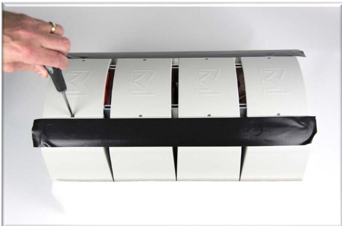
Take off the rear covers by removing the rear screws from each unit.
