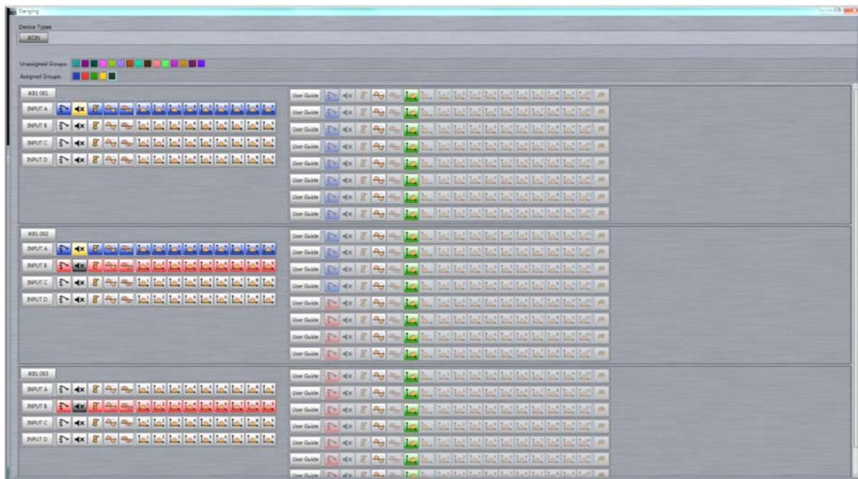
Once the system is configured to your satisfaction a Master Overview gives a complete picture of even the most complex system allowing you to monitor all metering and access commonly needed functions such as gain and mute.
