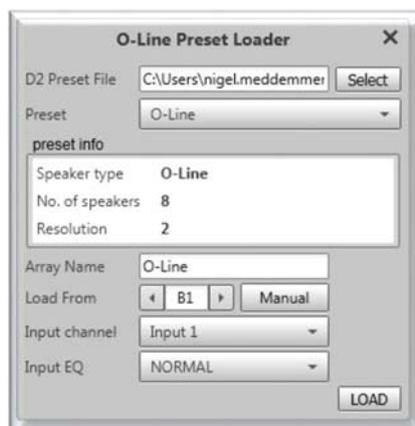
Click on 'Load' and the file is uploaded to the amplifier and an icon of your array is added to the project. For a stereo system, repeat the process selecting the next amplifier channel from which you need to drive the second array
