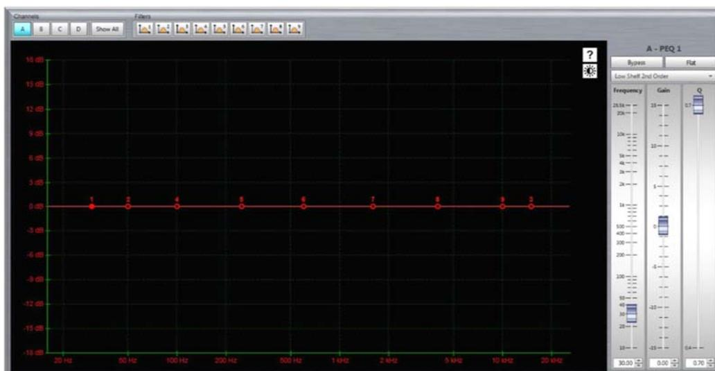
The output EQ is greyed out as it is used to apply the EQ created by your Display project, however the high pass filter is available for adjustment so you can determine the crossover point between the O-Line array and subwoofers if used.
