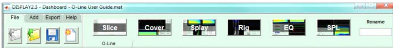
First a 2D slice of the venue is created, the coverage within the venue is specified, the splay angles calculated. A rigging report allows you to deploy the array and whilst that is being done the EQ coefficients are calculated. Finally an SPL report gives detailed information showing exactly how the system will perform. The computer model is accurate to within +/- 1dB of actual measured results so the SPL tab is a reliable overview of how well your system design will cover the space.
