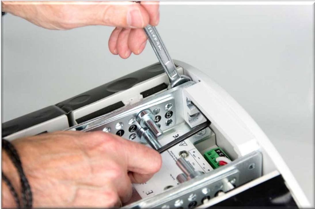
*Tighten the fixing nuts and bolts*
