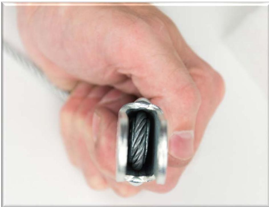
Loop the wire round the wedge and pull it semi-tight.
