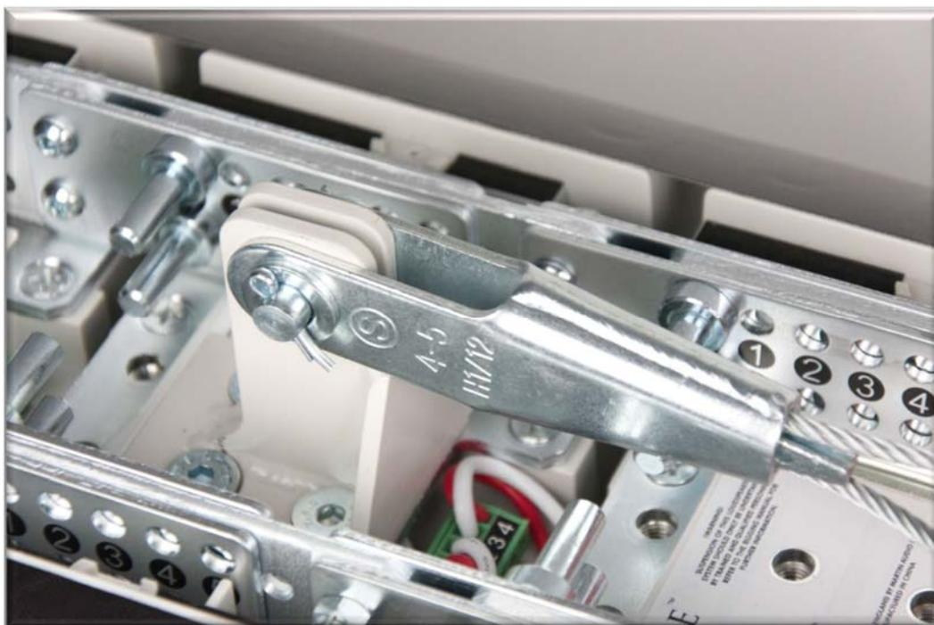
Roughly adjust the length of the wire using the wedge socket.
