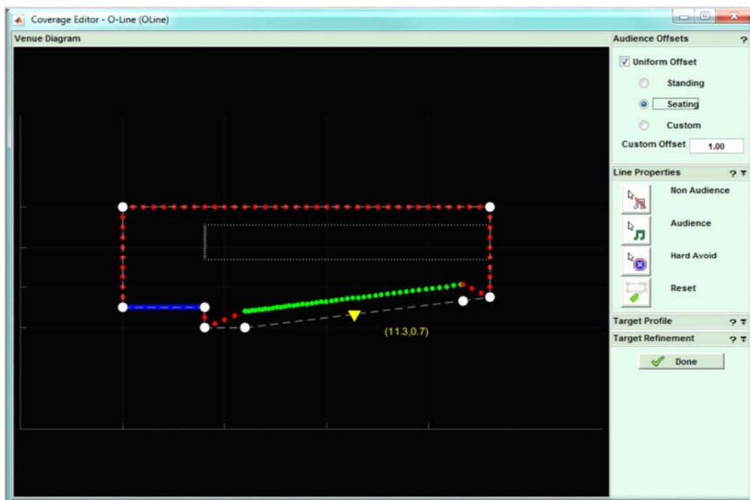
The coverage tab shows your 2D model with the planes refined into three types;-audience in green, non-audience in red and hard avoid in blue. Each dot represents a virtual microphone position at which the software will take response measurements using the integral computer model. The dots in the critical audience region are closer together for greater accuracy and are spaced closer together at the start of the audience region to mirror how each region is covered by sections of the array. The
