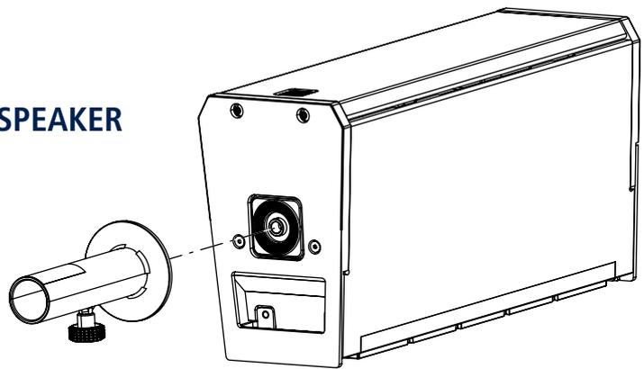
Once the pole mount kit is strongly tighten to the speaker you can mount it on a speaker stand or over a subwoofer.
