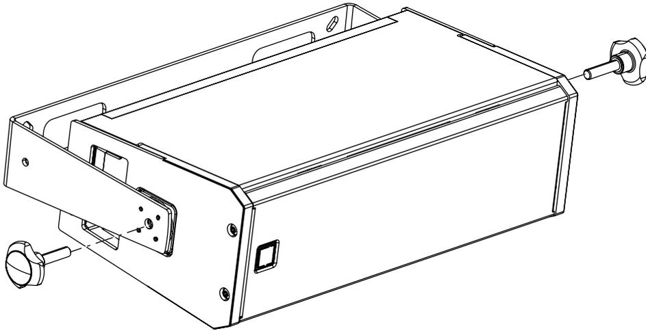
To change the inclination, loosen the knob or bolt and tilt the speaker. Once chosen the desired inclination tighten strongly the knob or bolt.
