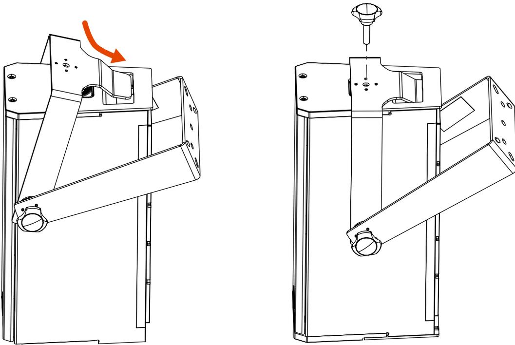
To change the inclination, loosen the two side knobs or bolts and tilt the speaker. Once chosen the desired inclination tighten strongly the two knobs or bolts.
