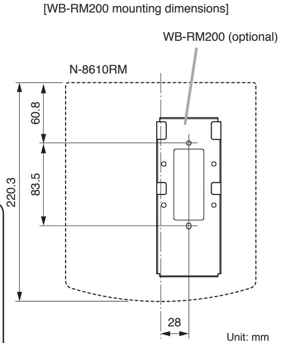
**Step 2.** Hook the bottom surface of the N-8610RM onto the WB-RM200.
