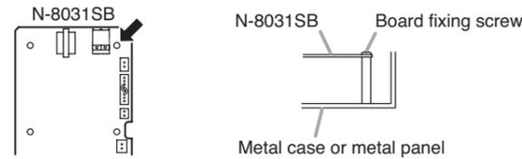
Cover the whole board with a case when installing.
