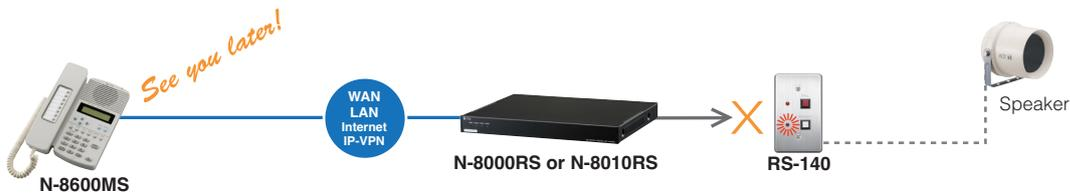
**Direct Select** Configures an operation panel equipped with indicator lamps and control buttons for the master station. Compatible with other stations, the panel assigns the various contact input and output channels to the master station and substations for purposes of identifying which substation is calling the programmed master station.
