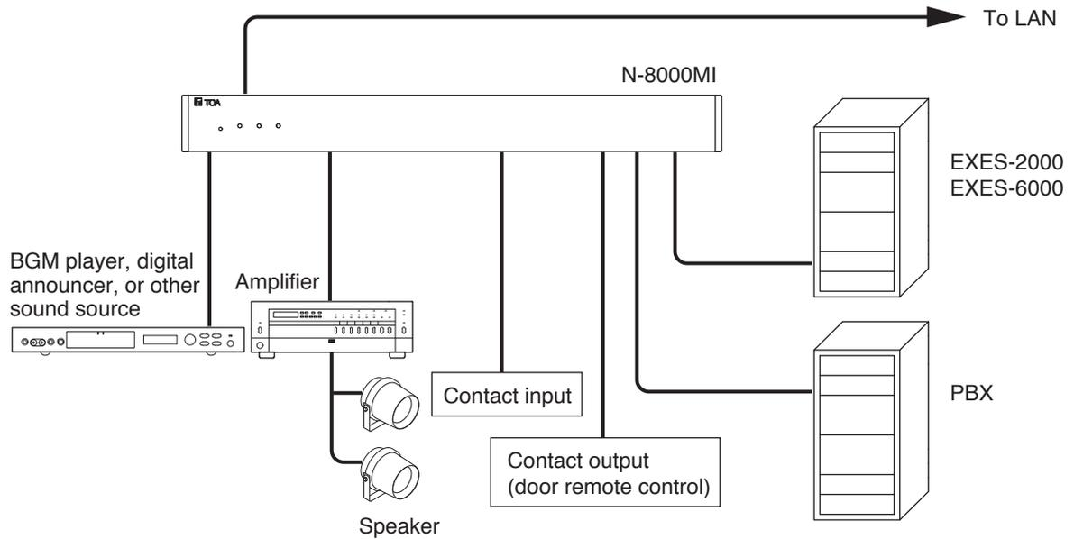
Having 2 channels each for audio input and output, and 16 contacts each for control input and output, the N-8000MI performs the following interface functions\*.
