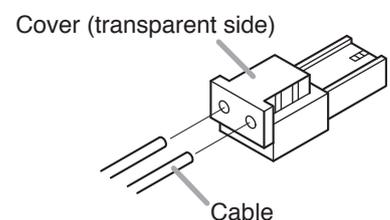
**Step 2.** With a pair of pliers, lightly pinch the mini-clamp cover and, after ensuring that the cable is securely inserted, firmly squeeze on the cover.
