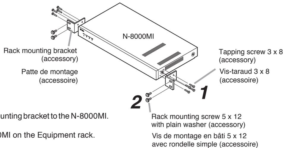
**Step 1.** Install the rack-mounting bracket to the N-8000MI.
