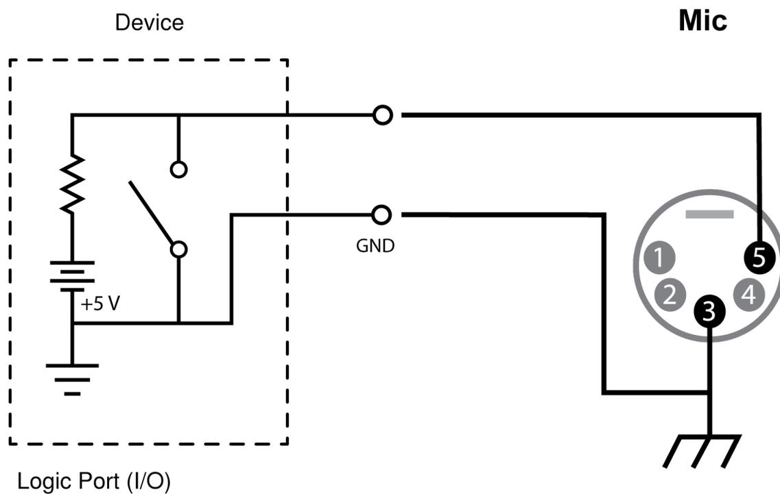
Connection to device with internal "pull-up resistor" logic circuit
