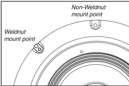
2.) Next, using 4 pcs - #10 x 0.75 in (19mm) sheet metal screw, attach the baffle / driver to the back can. Be sure to match the mounting holes without weldnuts to clipnuts on back can.
