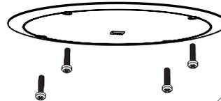
4 pcs - M4 x 38mm powder coated machine screws for attaching the metal grille to the baffle. (Included with JBL Professional grilles.)
