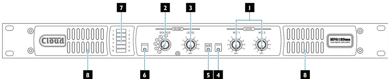
1. **MIC 1 and 2 LEVEL** – level controls for Mic Inputs 1 and 2.
