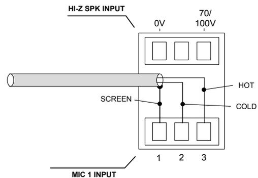
12 V phantom power is available at the mic input, and is activated by setting internal jumper J3 to the ON position. See page 25 for locations of internal jumpers. Care should be taken to ensure that phantom power is activated only when the microphone connected to the input requires it – i.e., a capacitor or electret type; other types of microphones (such as dynamic) may be damaged if a DC voltage is applied to them.
