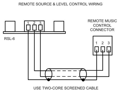
Use two-core (RSL-6 or RL-1) or single-core (RL-1 only) screened cable to connect the remote level plate (max length 100 metres).
