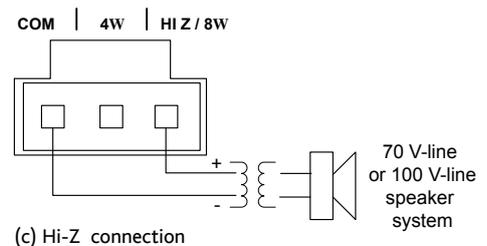
When driving 70/100 V-line loudspeaker systems there is a risk of transformer core saturation at high levels and low frequencies, which can produce distortion. To prevent this, the MPA MK2's output stage is provided with a 65 Hz high-pass filter, which may be enabled by setting **SPEAKER SETTINGS** switch SW1 to on (SWITCH down).
