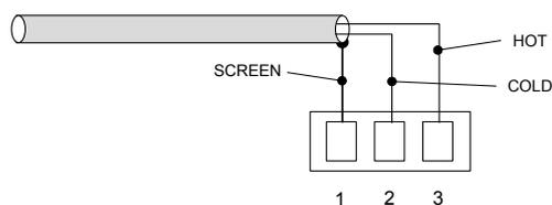
12 V phantom power is available at Mic input 2, and is activated by setting internal jumper J4 to the ON position. See page 25 for locations of internal jumpers. Care should be taken to ensure that phantom power is activated only when the microphone connected to the input requires it – i.e., a capacitor or electret type; other types of microphones (such as dynamic) may be damaged if a DC voltage is applied to them.
