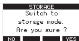
3. To connect with the computer, press the **F4 YES** button. The unit enters USB storage mode and connects with the computer.
