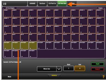
Use the I/O screen I/O Port Out tab to patch signals to the MMO card outputs. The port channels map to the MMO sockets as below.
