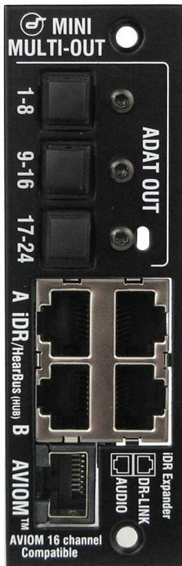
The **Mini Multi Out** (MMO) module is one of several plug-in card options that may be fitted to iLive **Port B** or the GLD I/O port. It provides three formats of multi-channel digital output simultaneously available for recording, personal monitoring and signal distribution.
