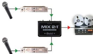
**Mix the output of two preamps to a single track**
