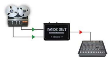
**Summing a stereo source to a single channel on a console**
