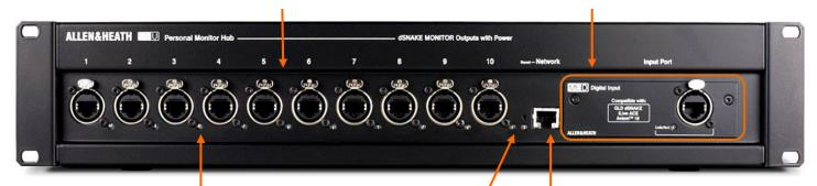
An indicator next to each port lights yellow to show it is linked to its connection, and flashes to show network activity. It lights red during start up or when an error is detected.
