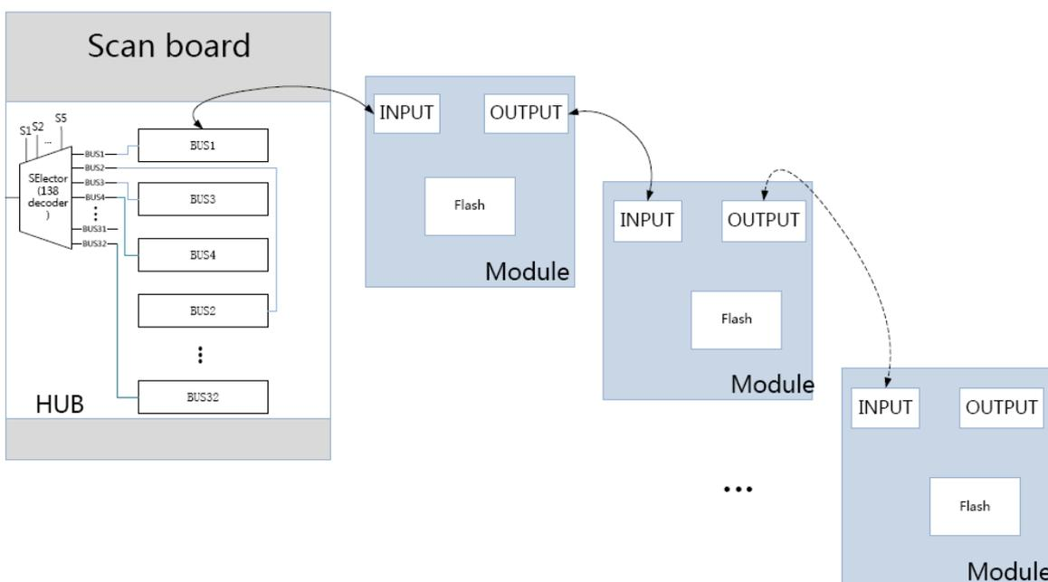
Fig. 5-27 Physical connection schematic diagram of Flash
