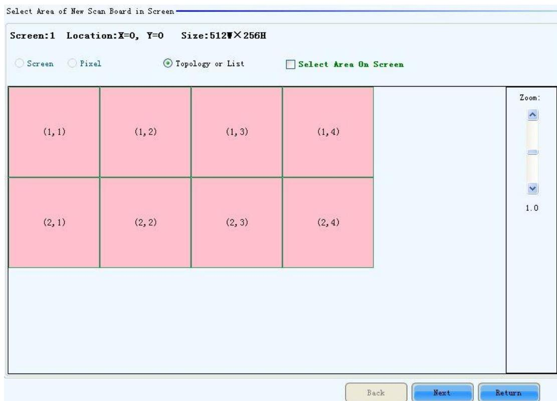
Fig. 5-88 The page for specifying the working area of the new receiver card
