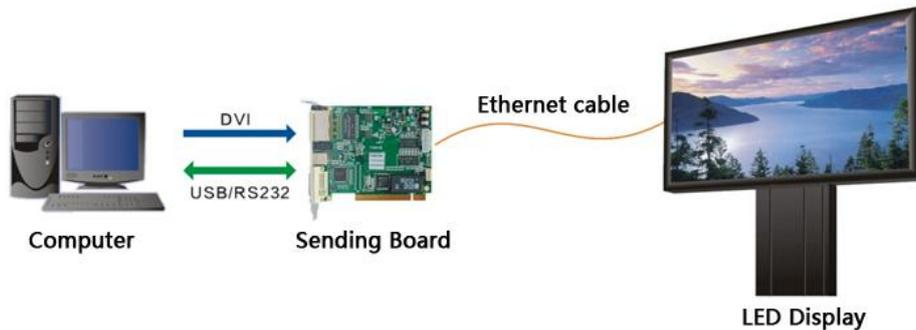
Fig. 1-1 Diagram of system architecture
