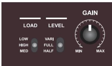
Set both 3-position switches to their middle position. This will disengage the GAIN control and provide maximum boost to your mic signal, while setting the load to a good starting point for experimenting.
