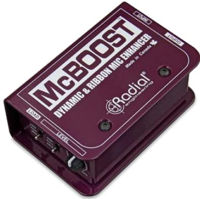
The Radial McBoost™ is a microphone signal booster designed to elevate the output of a typical dynamic microphone for greater transient response and boost the signal of a low-output ribbon mic to bring it up to a usable level for mixing consoles, preamps and workstations that may not provide sufficient gain. It features a 100% discrete class-A dual-transistor J-FET circuit that can produce up to 26dB of gain without introducing noise, color or artifact.
