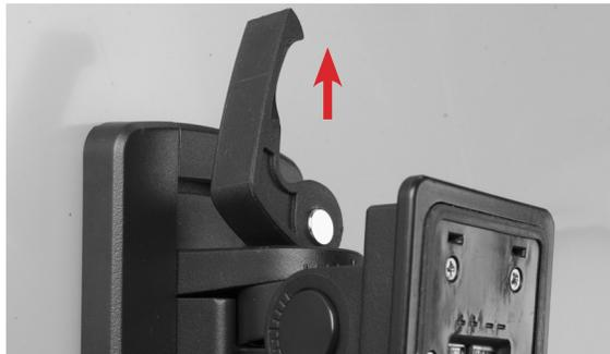
9. Attach the SAFCAB cable from the rear of the speaker to a secondary mounting point on the wall. Position the secondary mounting point close to and above the ClickMount to avoid kinetic force if the mount should fail.
