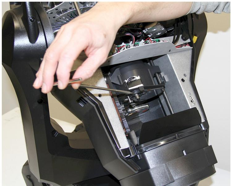
Figure 27: Unfastening the frost filter from its shaft
