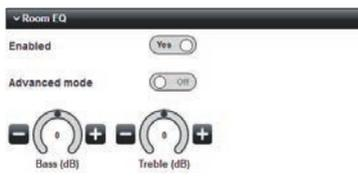
In Basic mode, simple treble and bass shelving filters are provided. The controls have a range of +/-12 dB at frequencies of 10 kHz and 50 Hz respectively.
