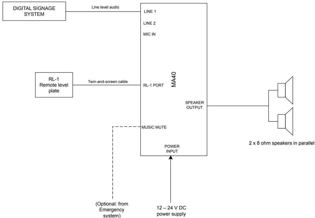
Video displays used in digital signage systems do not normally incorporate loudspeakers, and if they do, audio quality is frequently poor due to size constraints. The system shown here uses an MA40 to improve the audio in a digital signage system. The compact size of the MA40 makes it practical to attach it by some simple means to the rear of the displays themselves.
