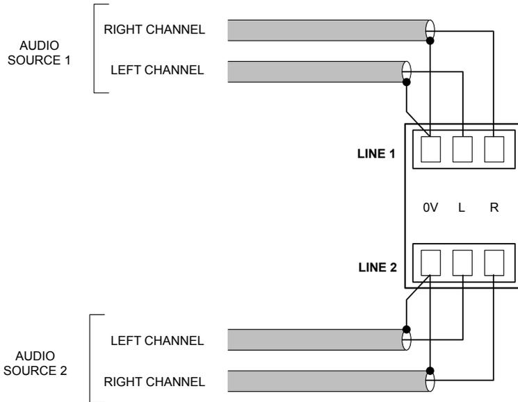
The two line inputs are summed together internally, though Line input 1 can be configured to have priority over Line input 2, see “Line 1 Priority” on page 18.
