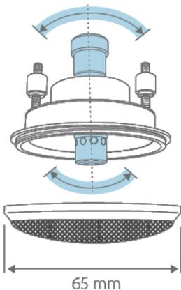
Audix's patented swivel mounting system can be rotated in any direction and angled up to 30 degrees toward a sound source.
