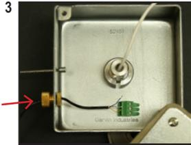
Insert plenum wire through strain relief nut, then connect to the Phoenix terminal.
