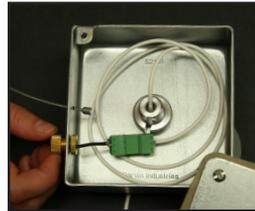
Tighten the strain relief nut.
