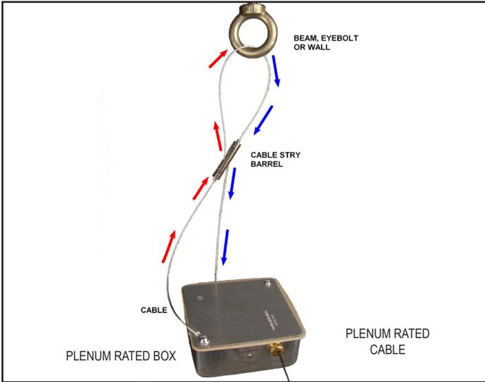
Wrap the cable around a beam, eyebolt or hanger. Next, slip the cable through the top of cable stay barrel pulling excess cable until taut.
