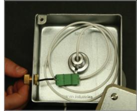
**6.** Tighten the strain relief nut. Arrange excess wire in box and fasten lid.
