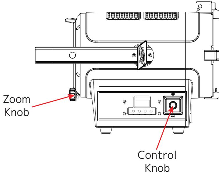
**ZOOM KNOB:** Manually adjust the zoom of the fixture in and out.
