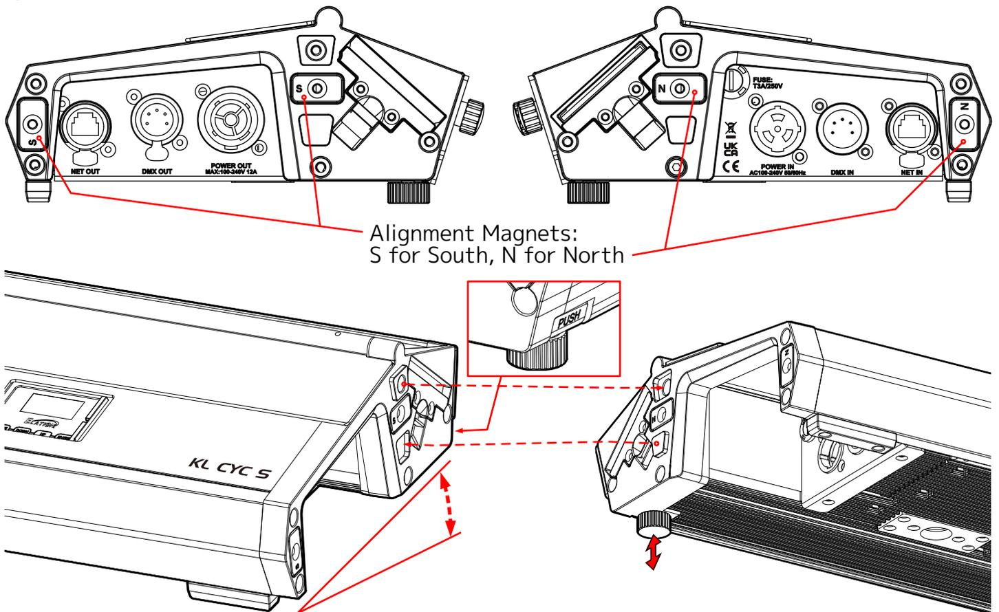
The corollary alignment features of the fixture, magnets, projections, and cavities, are designed to interlock when placed adjacent to each other with the same orientation. The front of the fixture can be raised or lowered to match these interlocking features, or to adjust the projection height of the fixture.
