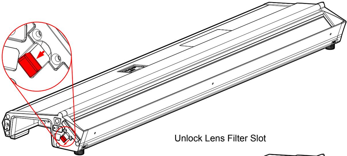
Unlock Lens Filter Slot
