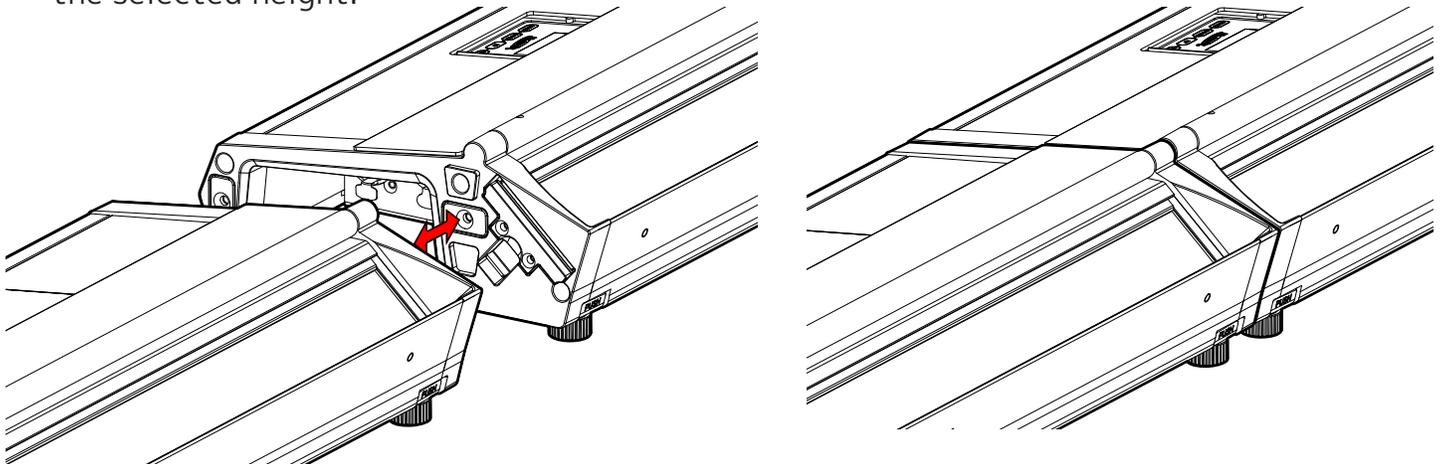
With the heights of adjacent fixtures adjusted to a matching height, orient the alignment features and move them together to allow their magnets to connect them and maintain their relative positions.
