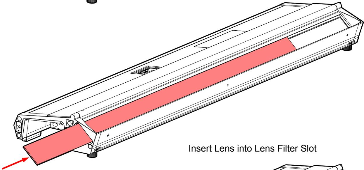
Insert Lens into Lens Filter Slot
