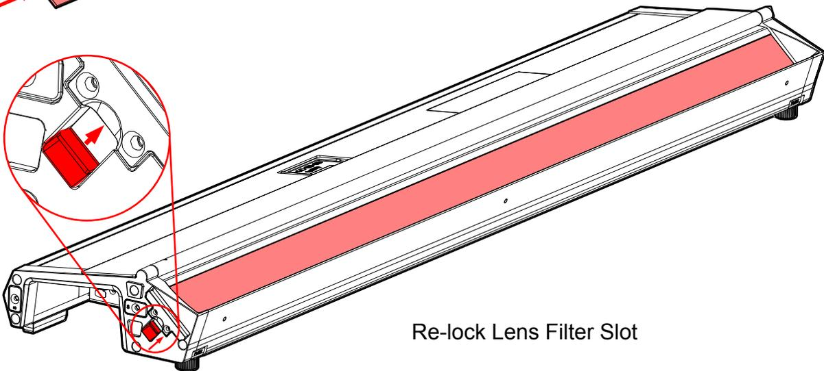
Re-lock Lens Filter Slot
