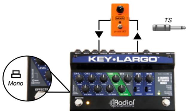
For stereo pedals and effects, make sure that the recessed Effects switch is disengaged. Use insert cables wired with 1/4" TRS to 2x 1/4" TS connectors to connect the SEND jack to the left and right inputs of the effects unit, and use a second insert cable to connect the outputs of the device to the TRS RECV connector on the Key-Largo.
