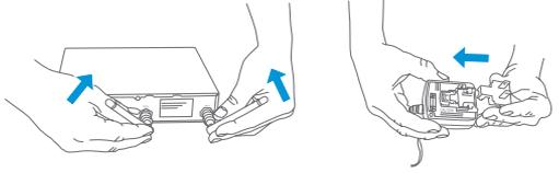
**3.** Plug in lavalier microphone, headset mic, or guitar cable into bodypack transmitter and secure by gently tightening the locking ring (if applicable)
