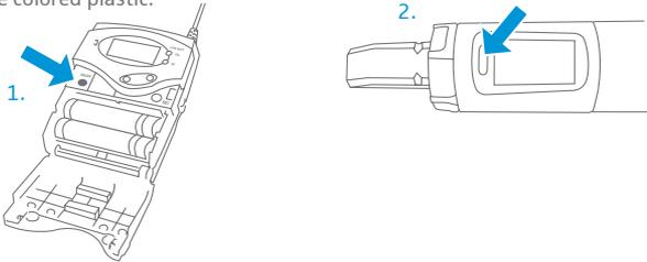
**5.** Enter SYNC mode by pressing "SYNC" button (EM receivers) or selecting SYNC option from menu (EK receiver). Once the SYNC logo displays, hold the handheld or bodypack infrared window facing the left side of the receiver display about 6" away. When SYNC is successful, you will see a check mark briefly next to the SYNC logo on the receiver screen. If you see an "X" next to the SYNC logo, it indicates the sync failed and you should repeat the SYNC process.
