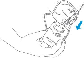
**4.** Insert 2 x AA (UM3) batteries into the transmitter (bodypack or handheld), observing polarity. (Camera sets only): Insert 2 x AA batteries into receiver bodypack (EK100G3). Connect either the 1/8" (3.5mm) or XLR camera output cable
