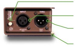
**INPUT PAD** Reduces input by 30dB to allow +4dB line-level devices to be connected.
