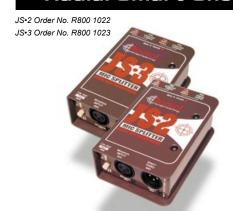
The Radial JS•2 and JS•3 are Jensen transformer-equipped mic splitters that allow a balanced source to drive multiple destinations via standard XLR connectors. These passive devices feature a premium nickel laminated core transformer for exceptionally low harmonic distortion without the usual phase shift caused by lesser steel core transformers.
