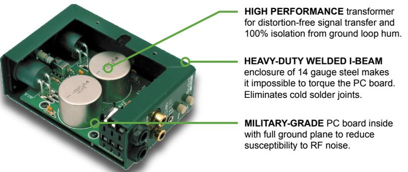
**HIGH PERFORMANCE** transformer for distortion-free signal transfer and 100% isolation from ground loop hum.
