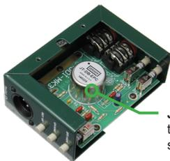
**JENSEN EQUIPPED** nickel core transformer provides distortion-free signal transfer and 100% isolation.
