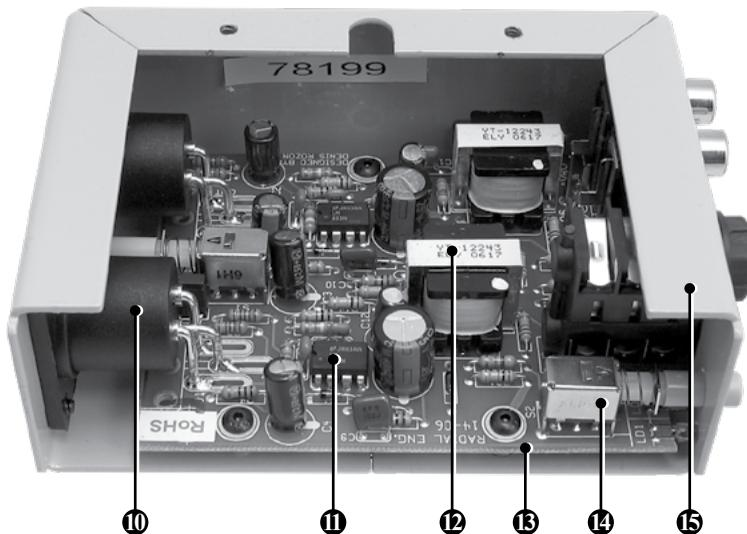
10. Isolated XLR connectors to eliminate chassis ground potential.
