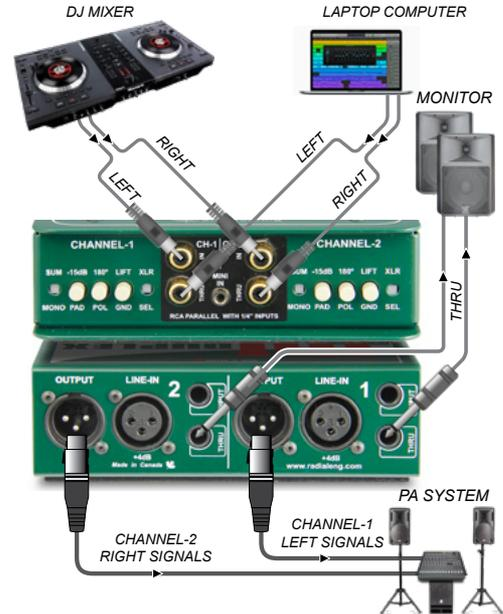
You may run into a situation where you need to take a +4dB balanced line-level source and convert it to a mic-level. This is particularly important in snake systems where the signal path is optimized for a microphone between -40dB and -20dB. If one were to connect a +4dB signal, the mic splitting transformers would likely overload and crosstalk would likely be introduced due to the +4dB line-level signal being significantly louder than the mic-level signal.
