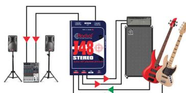
**J48 Stereo with two different instruments**
