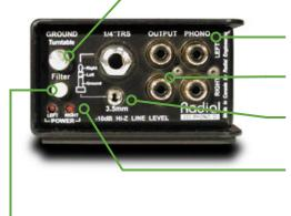
**THUMB SCREW** provides turntable ground connection to eliminate hum.
