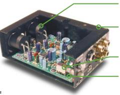
RUGGED glass-filled nylon connectors are 100% isolated for true dual-channel operation.
