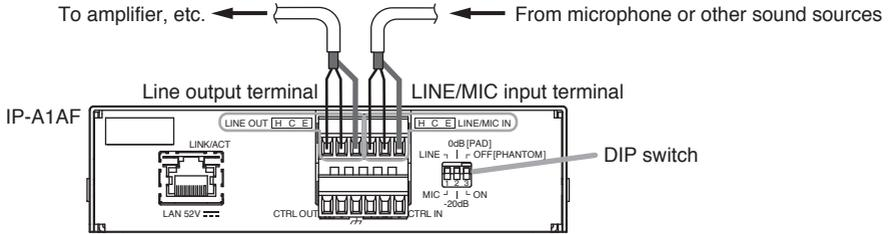
Set the DIP switch according to the audio device to be connected.
