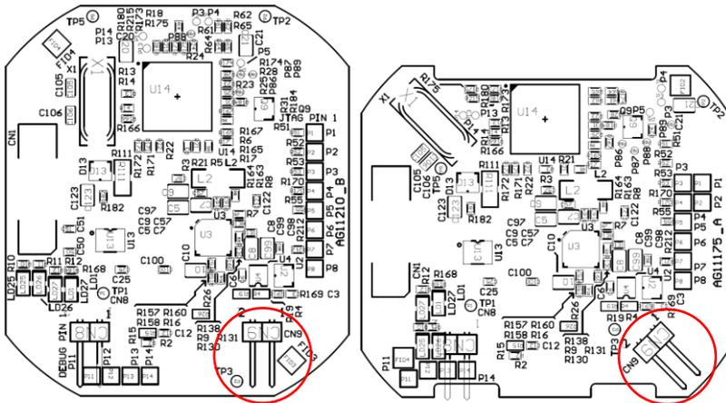
Jumper link **CN9** on the main PCB board lets you reset the network settings to factory default. To reset, short the link for 10s whilst applying power to the unit.
