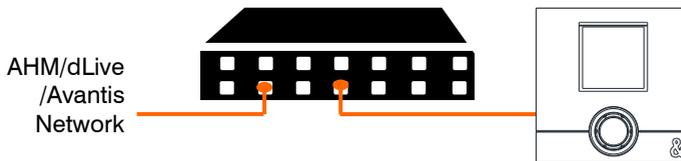
At power up, the unit Name and IP address are displayed on the LCD Display for easy identification of the unit. After a few seconds the IP1 will display level or function if any has been set for the unit.
