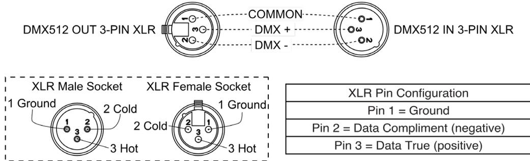
**Special Note: Line Termination.** When longer runs of cable are used, you may need to use a terminator on the last unit to avoid erratic behavior. A terminator is a 110-120 ohm 1/4 watt resistor which is connected between pins 2 and 3 of a male XLR connector (DATA + and DATA -). This unit is inserted in the female XLR connector of the last unit in your daisy chain to terminate the line. Using a cable terminator (ADJ part number Z-DMX/T) will decrease the chances of erratic behavior.
