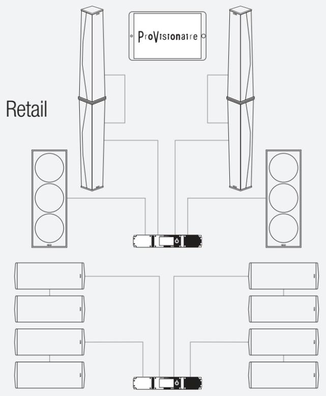
2 x ID84, 1 x IDS312 and 4 x ID24 per side, powered by NXAMP4X1MK2
