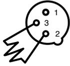
Termination reduces signal errors and avoids signal transmission problems and interference. It is always advisable to connect a DMX terminal, (Resistance 120 Ohm 1/4 W) between PIN 2 (DMX-) and PIN 3 (DMX+) of the last fixture. Figure 4
