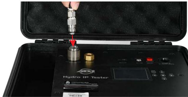
1. Connect the air hose quick-connect fitting to the Hydro IP Tester.
