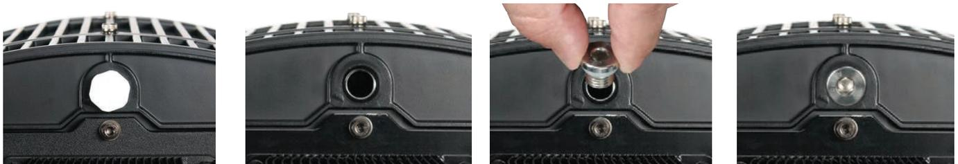
3. If the fixture has a second pressure relief valve, remove and replace it with an M12x1.5 Hex Socket Cap Head A4-70 Stainless Steel Bolt/Washer (included), and tighten using a 6mm Hex Wrench. *NOTE: Make sure the bolt has its O-ring for a proper seal.*
