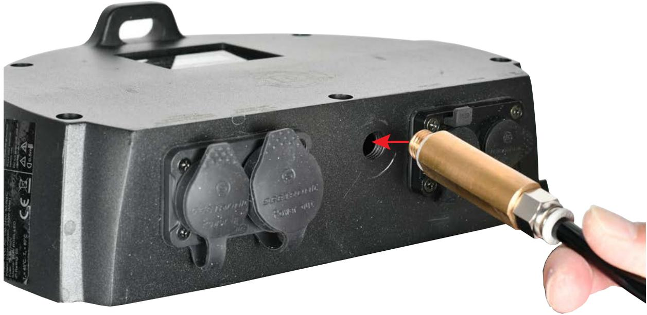
4. Carefully insert the threaded end of brass nozzle into the fixture air relief valve hole and twist it until it is finger tight and slightly compresses the rubber O-ring seal.
