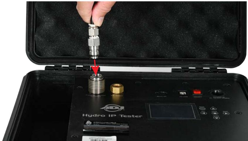
1. Connect the air hose quick-connect fitting to the Hydro IP Tester.
