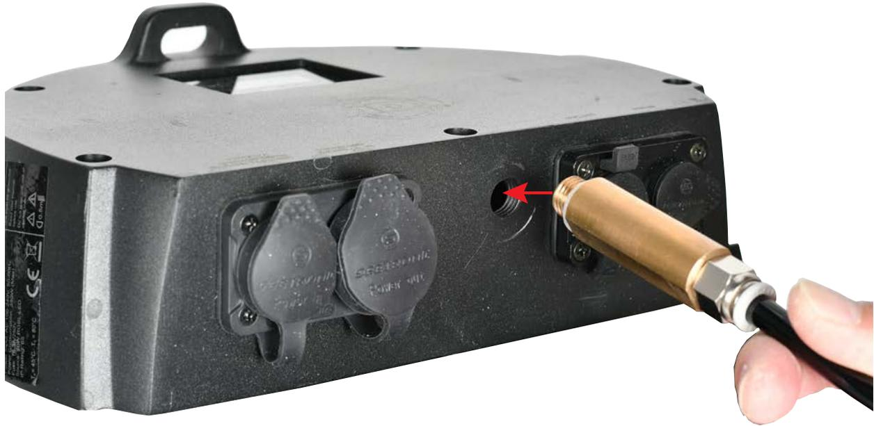
3. Carefully insert the threaded end of brass nozzle into the fixture air relief valve hole and twist it until it is finger tight and slightly compresses the rubber O-ring seal. *Make sure not to over tighten the brass nozzle or nylon bolt!*
