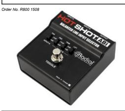
The Hot Shot ABi is a balanced line selecting device that lets you toggle between two sources and send the signal to a single destination. It features 100% passive operation with latching footswitch and therefore does not require any type of powering whatsoever. To add versatility both inputs are equipped with a -15dB pad and input B features a secondary -6dB trim to balance the two sources.
